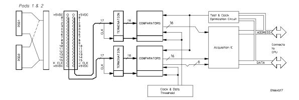
**The Main Circuit Board Logic Acquisition Circuitry**
